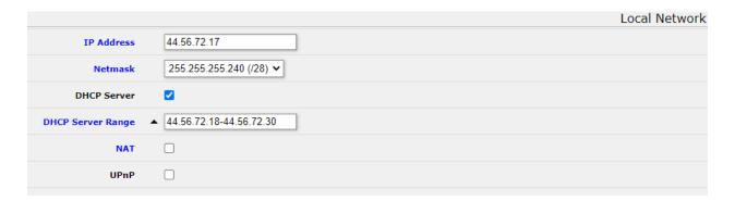
If you wish to use DHCP to dynamically assign addresses to your 44net devices, ensure that you enter the correct range of addresses in the "DHCP Server Range" field. A discussion on how to correctly identify usable IP addresses is without the scope of this document. If you are in any doubt please consult your allocation notice from your local sysop as in the below example.
