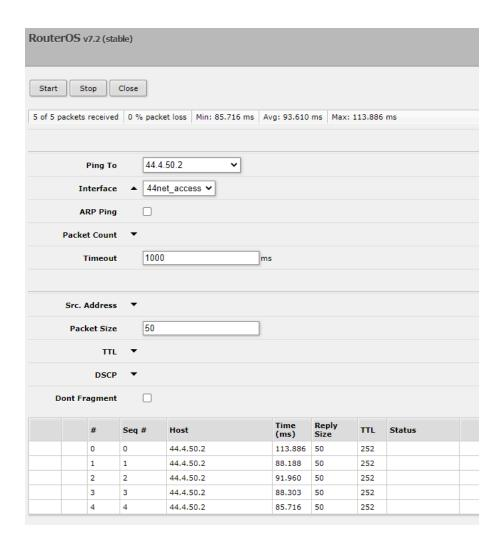
To test connectivity from your devices, issue a PING to 44.1.1.17 (portal.ampr.org). If this is successful, also do a traceroute or MTR to the same address. Your traceroute should reveal a handful of other 44net devices that your route passes along before arriving at the destination IP address. If you see public (non 44.x.x.x) addresses in the path then you may not be connected to the VPN. Check with your local sysop to confirm your connection status.
